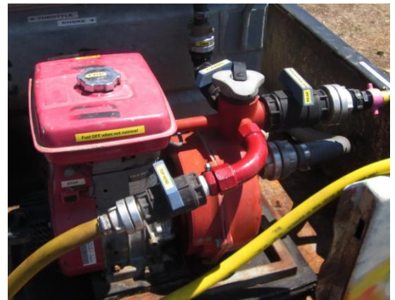
Pressure Pump - 3 outlets- cabin, top hose & blanket spray*
