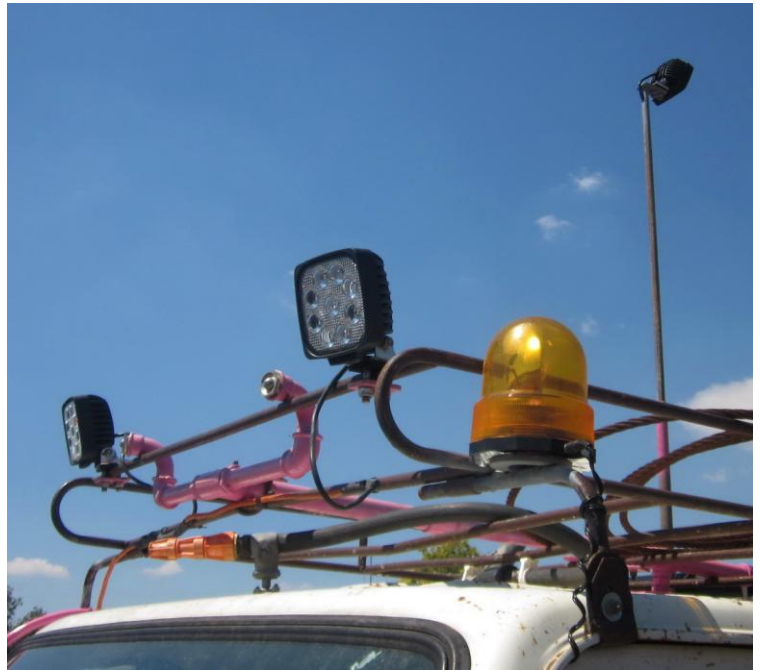
▲ LED work lights (2 forward & one extendable for the rear) Cabin operated hose with high flow multiple nozzles, Blanket spray system (pink piping)
