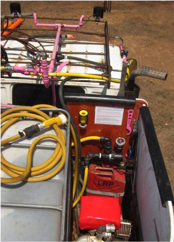
Hose operator station with heat shields ▲ and access to the blanket spray valve
