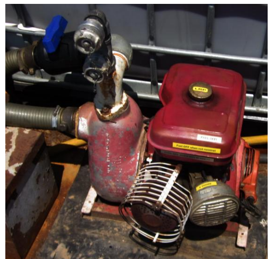
Quick-fill pump – used to transfer water from the forward tank to the rear tank as well as filling the complete unit in 5 minutes.
