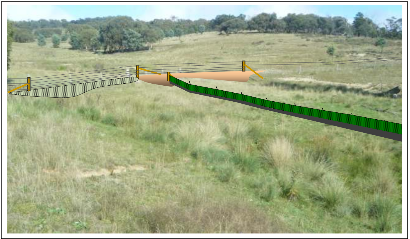
Upper diversion area with diversion bank. Stage 2.
